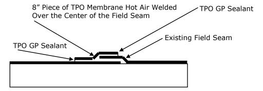
Note: The application of new TPO membrane to existing in-service TPO membrane requires special cleaning and priming procedures. Refer to Section F - "Cleaning and Priming of In-Service Membrane.
