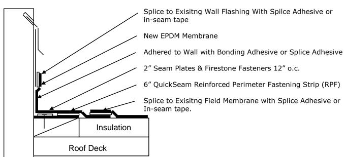
Note: The application of new EPDM membrane to existing in-service EPDM membrane requires special cleaning and priming procedures. Refer to Section F - "Cleaning and Priming of In-Service Membrane.
