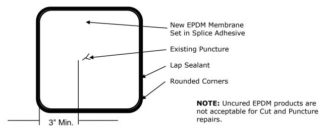
Note: The application of new EPDM membrane to existing in-service EPDM membrane requires special cleaning and priming procedures. Refer to Section F - "Cleaning and Priming of In-Service Membrane.
