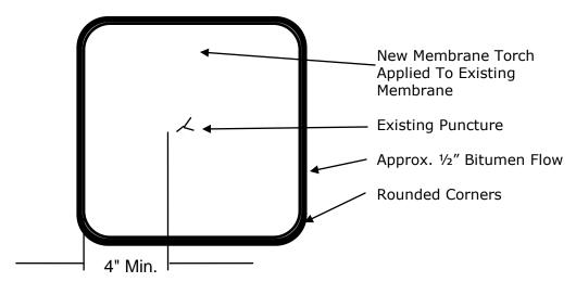
Note: Prepare existing surface by heating with a roofing torch and embed any exposed roofing granules and or lightly remove (without distorting the membrane compound) any applied coating with a heated trowel. After preparing the receiving surface and allowing to cool, apply primer to all surfaces receiving the new membrane patch.
