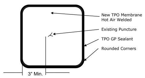
Note: The application of new TPO membrane to existing in-service TPO membrane requires special cleaning and priming procedures. Refer to Section F - "Cleaning and Priming of In-Service Membrane.
