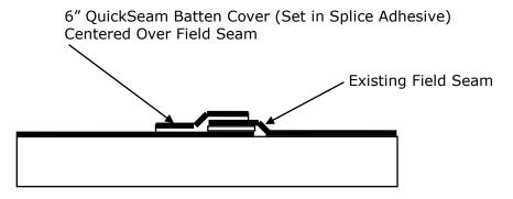
Note: The application of new EPDM membrane to existing in-service EPDM membrane requires special cleaning and priming procedures. Refer to Section F - "Cleaning and Priming of In-Service Membrane.
