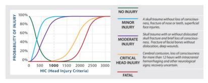
The above graph, which is included in ASTM F1292, describes the likelihood of injury in percentage points and the various types of injuries. It is important to note that at 1000 HIC (which is the maximum threshold), the probability for No Injury is 0%; the probability for Minor Injury is nearly 100%; and the probability for Moderate Injury is approx. 90%. Lower HIC measurements can significantly reduce the probability of injury.
