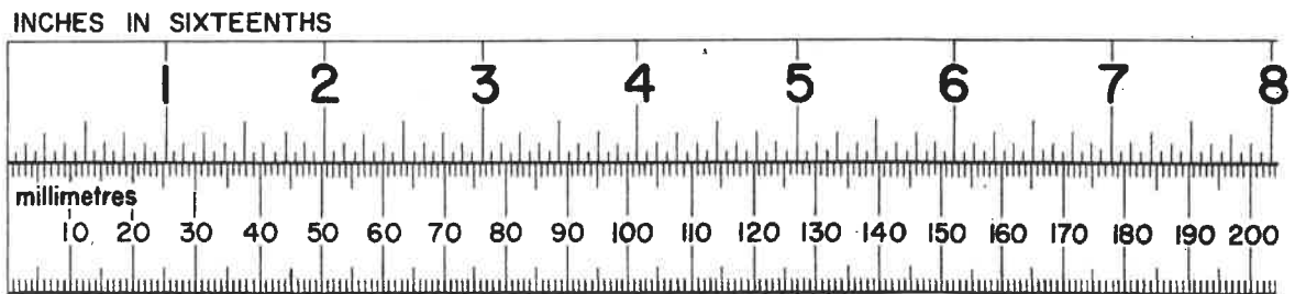
3-9. Customary rules are divided into inches and fractions of an inch. Metric rules are divided into centimetres and millimetres.
