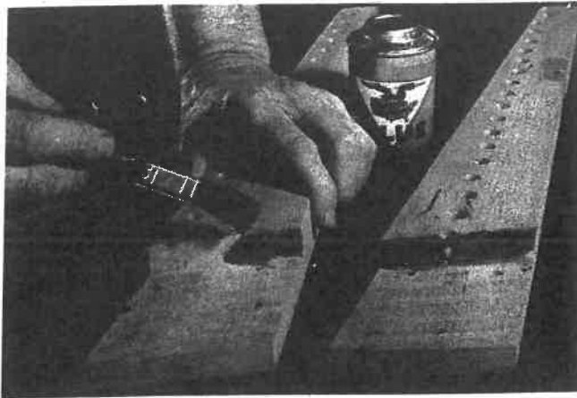
32-12. When gluing end grain it is a good idea to apply a thin coat of glue first. The end grain will absorb the glue. When applying glue to the rest of the joint, apply a second coat to the end grain. Notice that a brush is used to apply the liquid glue.
